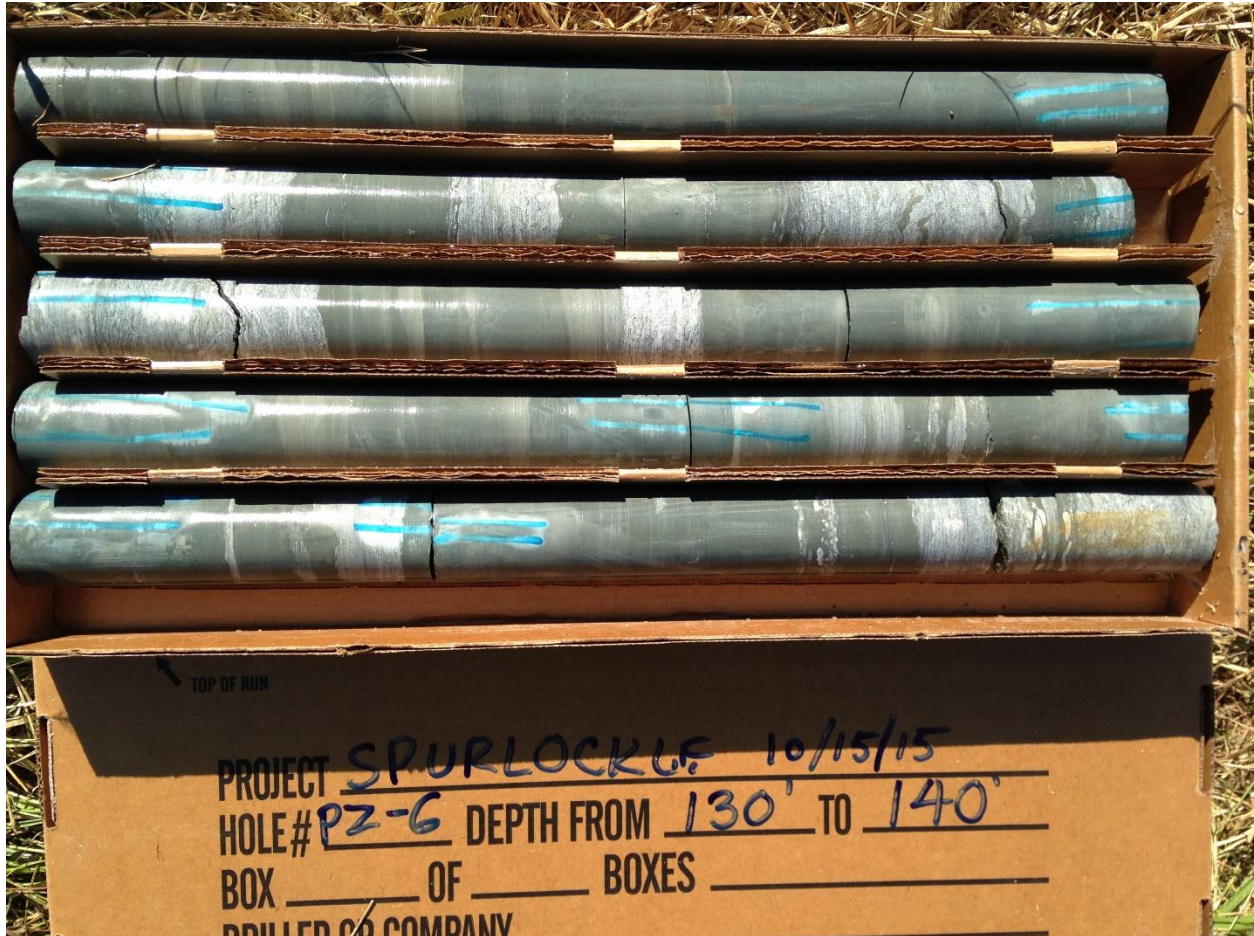
Figure 21. Photograph of a box of marked core from a 10-ft core run in the Kope and Fairview formations, showing mechanical breaks marked with blue-colored marker streaks. Core sticks like this would be included as portions of the core greater than 4 inches in length for determining RQD (photo provided by Kevin Carey).
