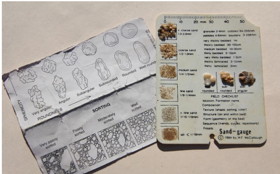
Figure 12. Illustrative guides or gauges for recognizing grain shape, grain size and sorting.
