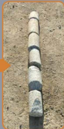
■ Granite core samples
