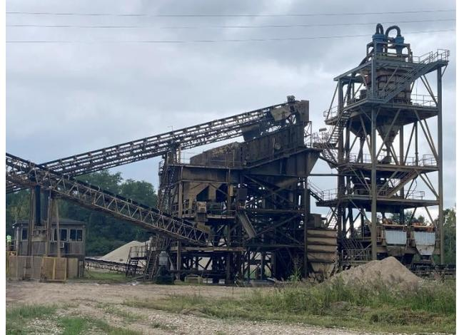
South view of sieve screen and wash assembly on left and density separator on right (STOP 2).
