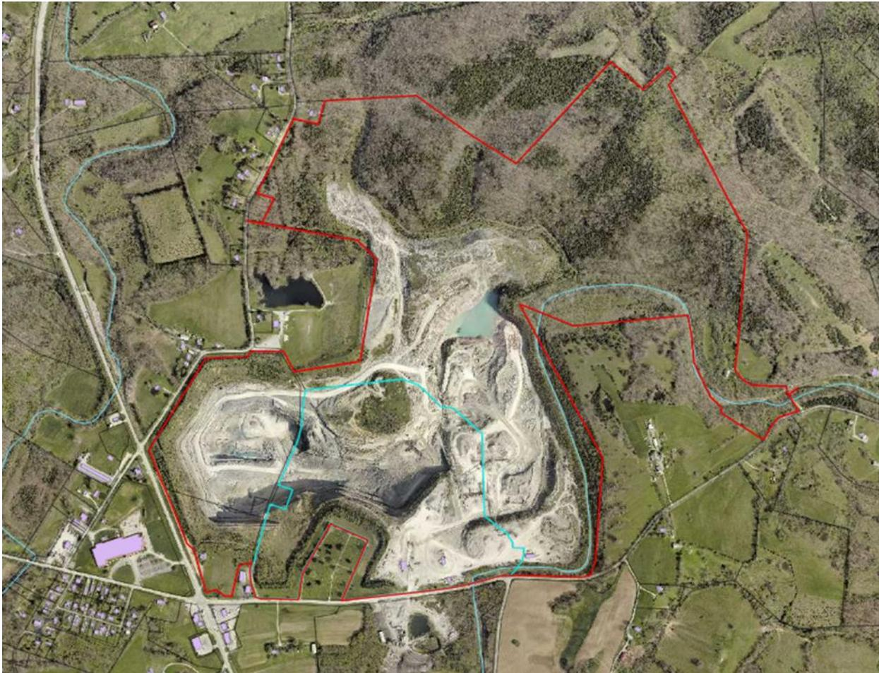
**Figure 11.** Pendleton County property tax map showing the location of the Butler Quarry and vicinity. The controlled property boundary (fee simple) is outlined in red colored lines and the mineral lease area is outlined in blue colored lines (Map Scale 1 in. = 0.25 mi.).
