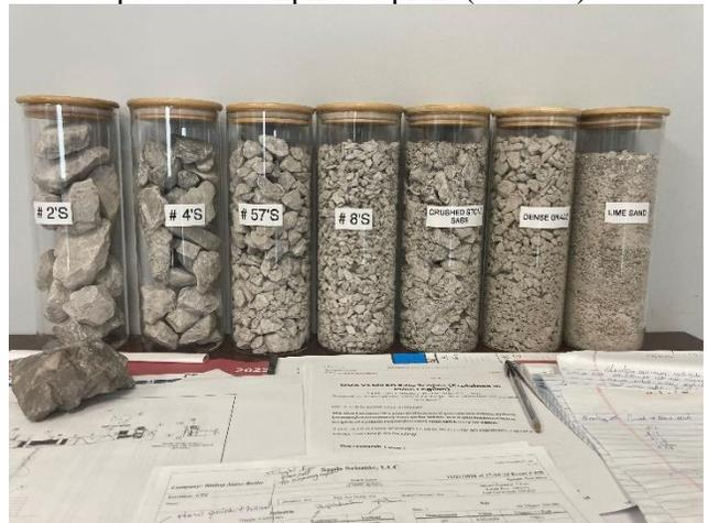
Photo of some of the sample size gradations produced at Butler Quarry (STOP 4).
