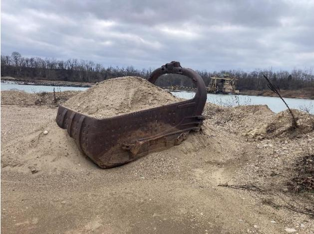
South view of 2-yard capacity fixed bucket dredge adjacent to pit (STOP 2).
